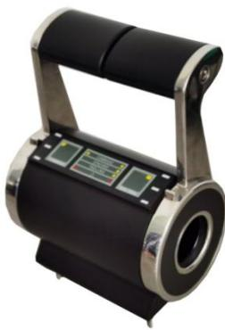
This is a dual engine controller/lever. Suitable for throttle control of twin-engine yachts, can control 2 engines, with throttle control, gear control functions. There are 3 mechanical gears DNR, synchronous indication. With Hall sensor, full temperature range linear compensation, 2 engines full electrical isolation technology, bus signal output and engine electronic throttle signal output, waterproof and anti-salt spray treatment, with good operating feel.
