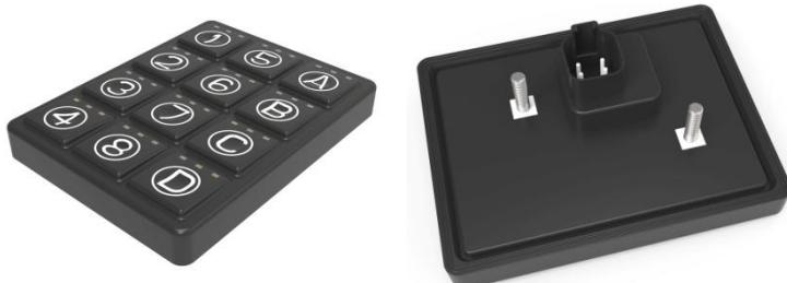
MKB-24N is a keypad with laser pattern. Each button has an etched pattern and colored backlight, and three adjustable brightness LED indicators provide diagnostic feedback that flashes if a malfunction occurs. The button panel is sealed and protected, and it can be installed inside or outside the driver's cab.
