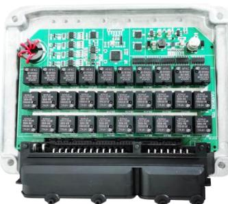
Function: Convert the switch signal from the CAN bus into a relay switch;
