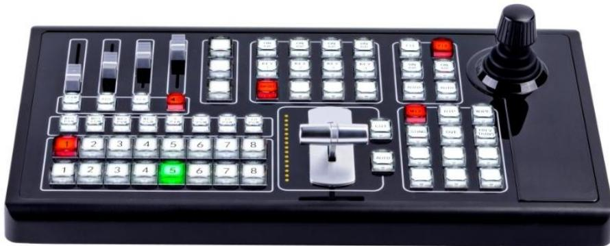
The video switcher is suitable for audio and video editing and live broadcast systems, recording and broadcasting systems. USB Hid, Midi protocol, support broadcast software such as vMix, support windows, macOS operating system, support RS232 interface communication, support RS422 camera control.
