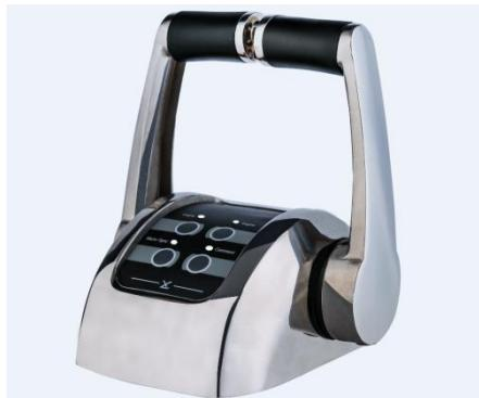
MKF-JS16 dual engine throttle controller. Suitable for ship engine throttle control, can control 2 engines, with throttle control and gear control functions. With CAN communication indication, synchronization indication, error indication function. Adopt dual-channel Hall sensor, full temperature range linear compensation, stainless steel shell, waterproof and salt spray design, friction resistance positioning, 3 mechanical gears (DNR).
