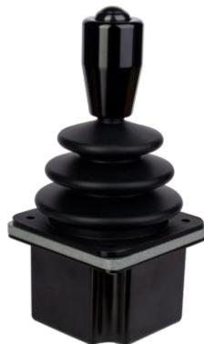
MKF-JS55 is a 2 axis Hall-type industrial joystick, instrument panel installation method, stainless steel and aluminum alloy materials, spring automatic return structure, German high-precision Hall-type sensor, full temperature range linear correction, IP65 protection level, smoother operation Feel, ergonomic mechanical design. reliable for long life span usage. This joystick is specially designed for rotary excavator and other heavy-duty or safety-critical applications.
