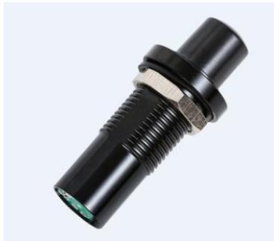
PB-12 series Hall linear buttons. The spring automatically returns; linear voltage signal output, 0V when the button is released, 4.5V when it is pressed to the end, linear signal output.
