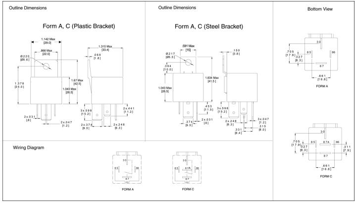
Dimensions in inches with millimeters in brackets below. Tolerance: ± .010"
