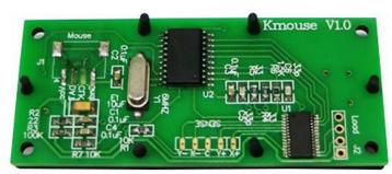
**Product Code MKB-1-FS** Mate Mouse, Silicone, Force Sensing Resistor, Panel Mounted
